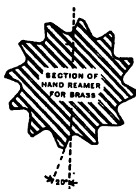
FIG. 19.—TEETH OF HAND REAMER WITH NEGATIVE RAKE.
